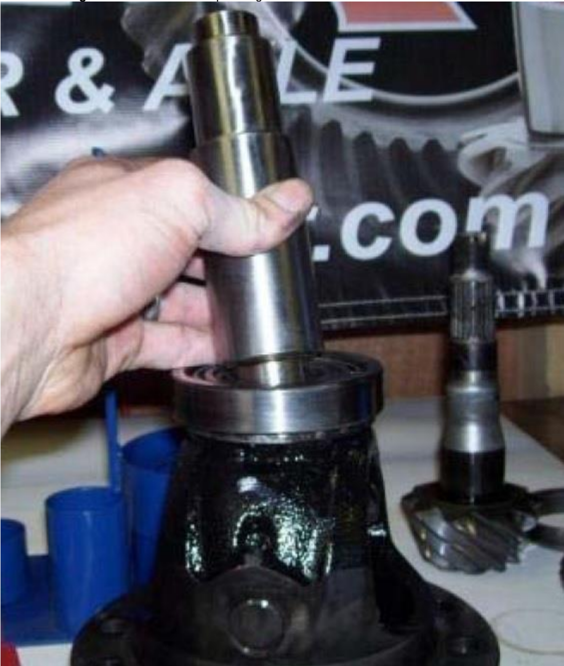
Place body of puller over adapter and screw bottom adjuster down onto race, slide clam-shell half on and screw top adjuster until it contacts clam-shell.
